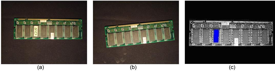
**Figure 8:** Result for a RAM Module. (a) Original sample, (b) damaged sample, (c) highlighted defects.
