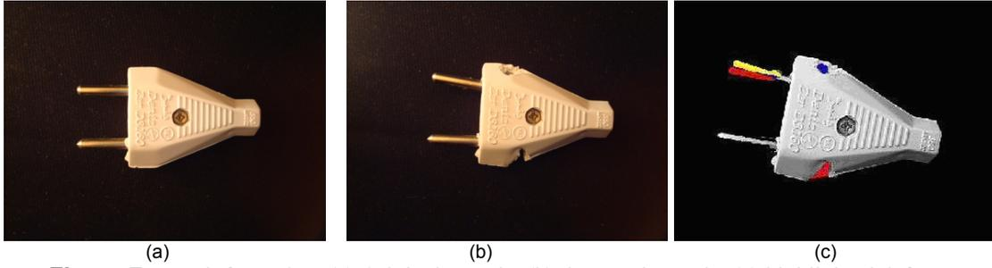
**Figure 7:** Result for a plug. (a) Original sample, (b) damaged sample, (c) highlighted defects.
