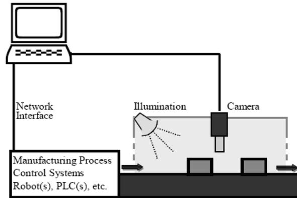
**Figure 3:** Hardware setup of proposed AVI system.
