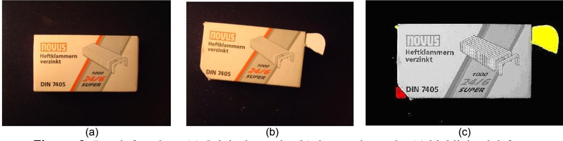
**Figure 6:** Result for a box. (a) Original sample, (b) damaged sample, (c) highlighted defects.
