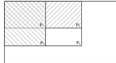
**Figure 2** – to compute sum of pixels in white box, subtraction of  $ii(p_4)$  from hatched section, that is  $ii(p_2)$  plus  $ii(p_3)$  minus  $ii(p_1)$ , should be computed.
