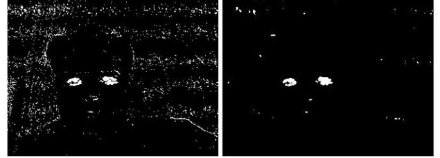
**Figure 3** – One pass Fast Median filter result. Left image is noisy threshold difference image and Right image is the result of Proposed Fast Median Filter.
