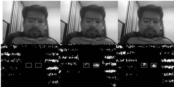
**Figure 6** – An example of blink detection. Blink is detected in last frame (right most images) and is highlighted in earlier frames.
